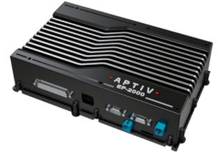
The EP-2000 runs Aptiv's Connect Edge software to detect anomalies and monitor when signals have exceeded configurable thresholds. These advanced triggering capabilities allow you to specify exactly which data you want to collect and when you want to collect it. It provides the rich, high-fidelity data you need for troubleshooting advanced vehicle systems.
