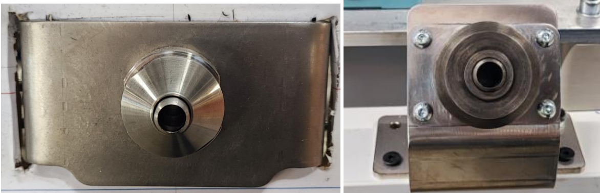
Rys. 5 – View of sample screen curling tools
