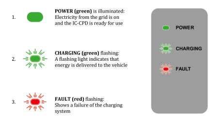
According to the operating mode, the IC-CPD charging equipment emits different combinations of continuously illuminated and/or flashing LEDs. (For additional explanations, see page 19)
