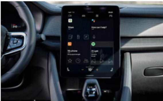
OEMs send updates and security patches automatically over-the-air to the vehicle’s telematics box. The customer receives a notification that an update is available, and, similar to what happens with a smartphone or laptop, the customer can select an upgrade option, such as performing the update while the vehicle is charging overnight.
