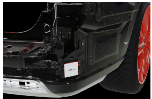
Figure 2. Radar can be located behind the outer body of a vehicle.
