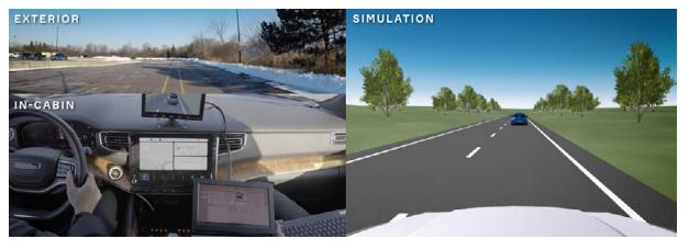
Vehicle-in-the-loop: In VIL, simulated inputs are fed to real hardware in a full vehicle.
