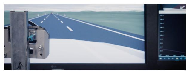
Hardware-in-the-loop: A HIL bench presents simulated inputs to real hardware.
