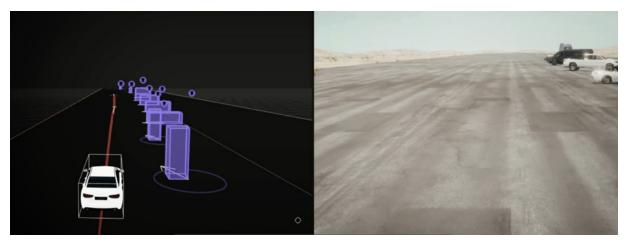
**Software-in-the-loop:** With SIL, simulations occur entirely in software.
