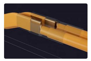
Welded interfaces can have issues as well, including improper bonding between the cable and the terminal. This could occur as a result of poor tooling and weld parameter setup, the
