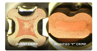
On AC charging circuits, mechanical crimps are more common, but they often don't get as much attention as they should. Bad crimps are a major cause of high resistance and excessive heat. Root causes include improper compaction, crimp relaxation over time and inadequate process control.
