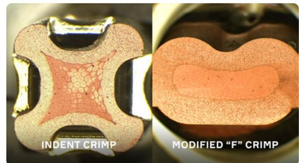
On AC charging circuits, mechanical crimps are more common, but they often don’t get as much attention as they should. Bad crimps are a major cause of high resistance and excessive heat. Root causes include improper compaction, crimp relaxation over time and inadequate process control.
