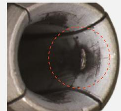
PLATING MAY NOT ADDRESS HIGH RESISTANCE CAUSED BY ARCING OR DAMAGED CONTACTS WITH LOW NORMAL FORCE
