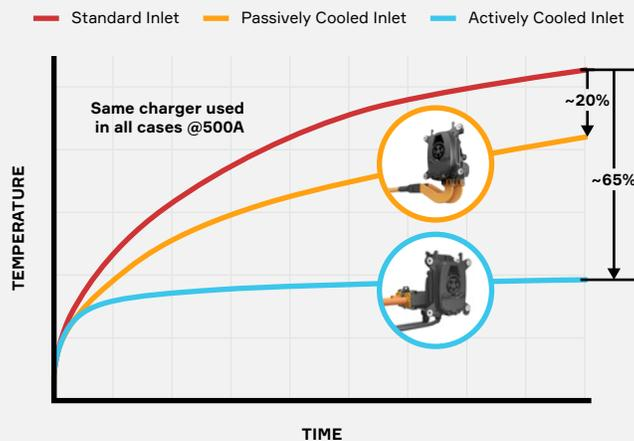
Temperature monitoring systems should be able to accurately track the true temperature of the terminals in real time, with minimal lag. This feature is critical because it allows the system to react quickly enough to rapid temperature increases and appropriately shut down or derate charging.
