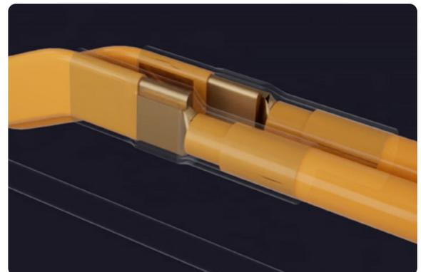
Welded interfaces can have issues as well, including improper bonding between the cable and the terminal. This could occur as a result of poor tooling and weld parameter setup, the
