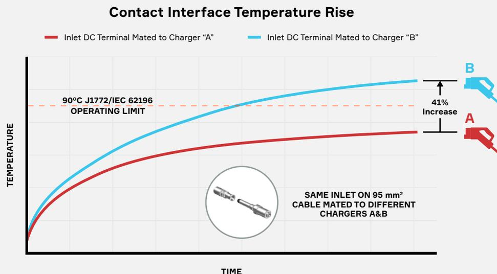
High temperatures observed as a result of differences in contact interface resistance and thermal management systems
