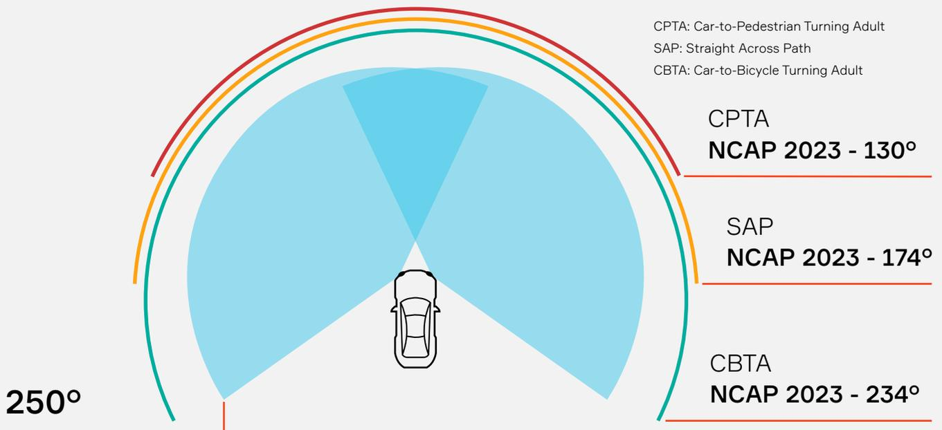
Taken together, the two front corner radars provide 250 degrees of perception with all of radar's strengths. Radar provides strong distance and speed detection through a wide range of environmental conditions – including harsh weather, poor lighting and heavy dust and dirt – while also allowing OEMs to package the sensors behind fascia and in tight spaces.
